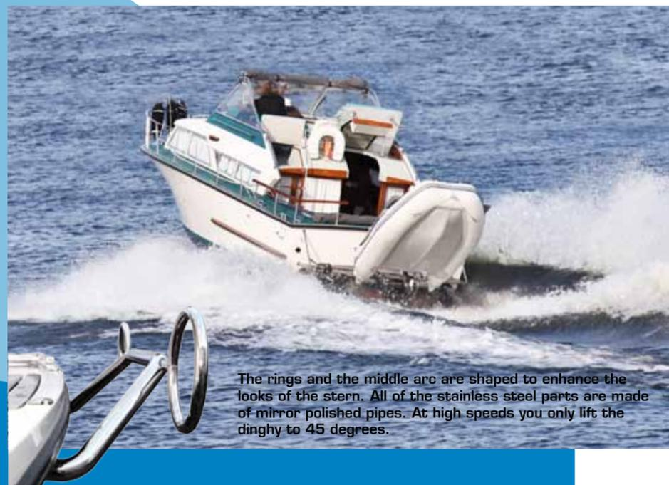
The rings and the middle arc are shaped to enhance the looks of the stern. All of the stainless steel parts are made of mirror polished pipes. At high speeds you only lift the dinghy to 45 degrees.
