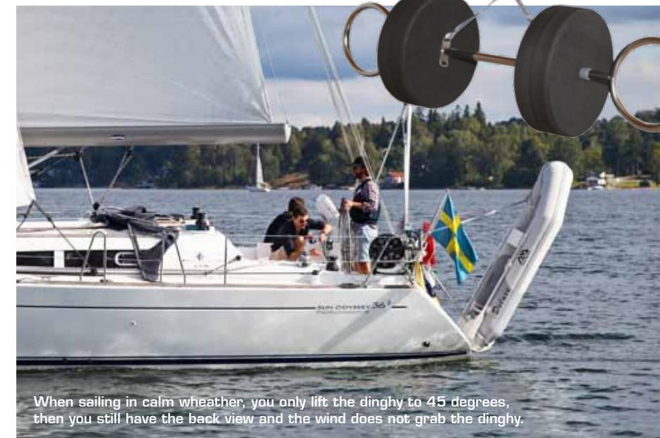
When sailing in calm weather, you only lift the dinghy to 45 degrees, then you still have the back view and the wind does not grab the dinghy.
